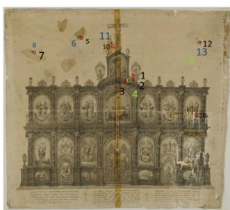
Figure. 1: micro-XRF spots, line and area scan measurements on printed silk scarf Temple of the Holy Trinity Greek Orthodox Church of Vienna Printed Silk Scarf, 1822-1858 Vienna (566mm width x 633mm length) ©National Historical Museum of Greece NHM Import directory number: 11498.
